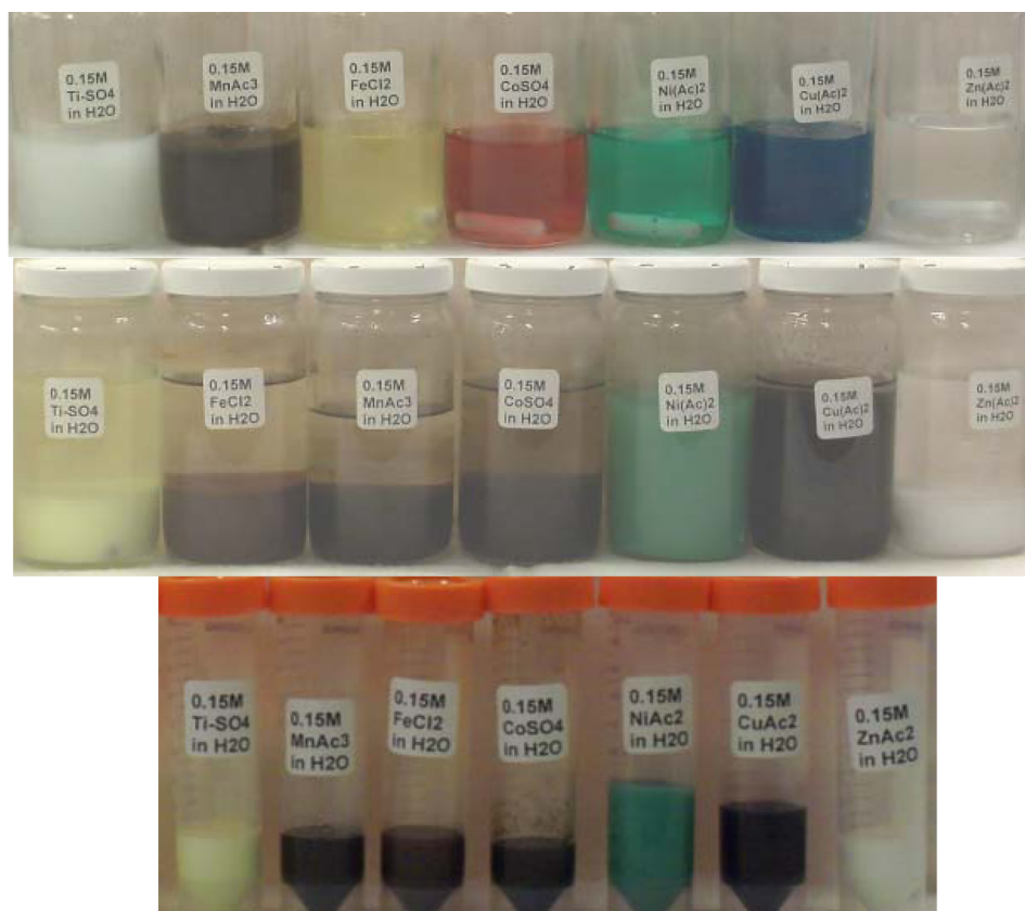
Figure 1. Illustration of the overall synthetic process: top row, simple salt solutions; middle row, solutions after the addition of \text{KO}_2 ; bottom row, the final nanoparticulate products.
